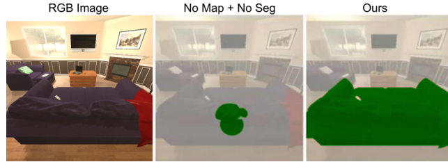
Fig. 4: An example image of the annotation approach used by [10] and the No Map + No Seg ablation (middle) compared to our approach which uses object segmentation and is therefore able to annotate the full object (right). Annotation masks are shown in green.
