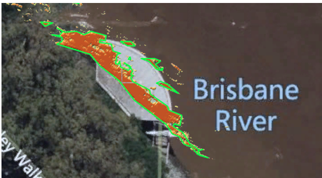
Fig. 5: Obstacle registration from a noisy occupancy map.
