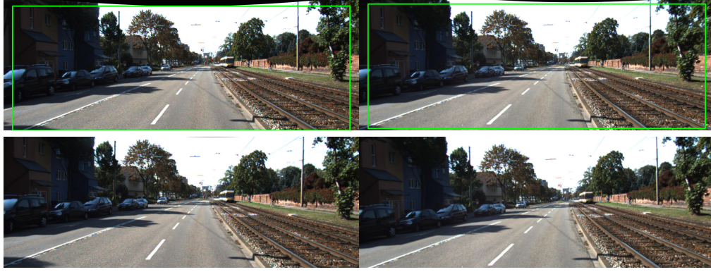
Fig. 1. Example of a rectified stereo pair with true calibration parameters from the KITTI dataset [23]. Top: Validity mask \mathcal{R} (green) corresponding to the largest rectangle containing only valid pixels with same aspect ratio as the original image. Bottom: Valid region after cropping and resizing to original image size as final input into the network
