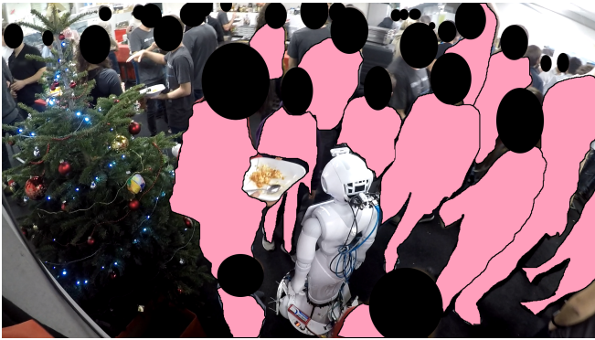
Fig. 3. Crowd density during the unstructured crowd experiment. Interested, unaware participants are obstructing the robot’s path. Nevertheless, the robot was able to reach its goal by using our assertive ‘nudge’ behavior.
