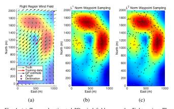
Fig. 1: (a) True and estimated 2D wind field across the flight region. The gradient of the estimated wind field is given by the underlying surface plot. A set of 200 random waypoint samples drawn from the (b)  $L^1$  norm and (c)  $L^2$  norm gradient distributions. Samples are shown as circles.
