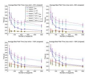
Fig. 2: Fastest time to travel from the origin node to the destination node across the four tested wind fields averaged over 100 random waypoint generations. 7 PRMs were tested, using either uniform or biased random sampling to select waypoints, and either a constant connection radius, defined as the lower bound of the PRM\* radius in (1), or a variable connection radius, computed from (4), to connect the waypoints in the graph.
