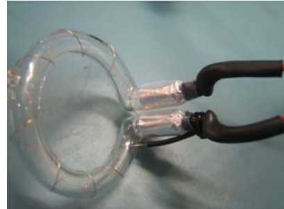
Figure 7: Trigger electrode for flash lamp
