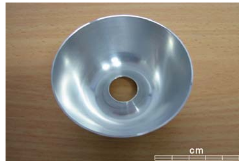
Figure 8: Spun aluminium reflector prior to polishing
