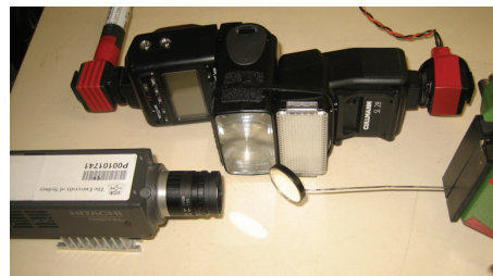
Figure 5: Proof of concept hardware for the collocated strobe and camera
