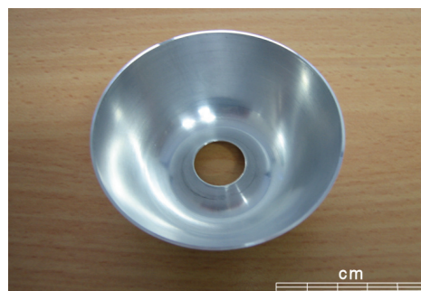
Figure 8: Spun aluminium reflector prior to polishing
